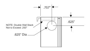
Low Version for use with Sashes that have Double Wall for Sash Lock screw insertion.
