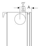
Mark over from front of sash A dimension plus .243". Mark Spot and Bore .625" dia  $\times$  .500" Deep Hole.
