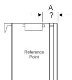
Measure from Flat Side of Tilt Latch engaging Jamb to Front Side of Sash.
